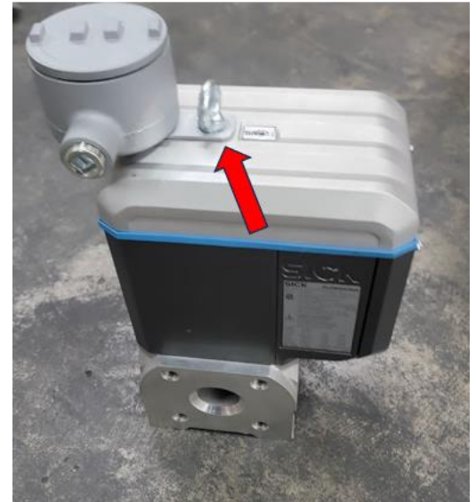
Example of mounting to flow meter using integral picking-eye.
